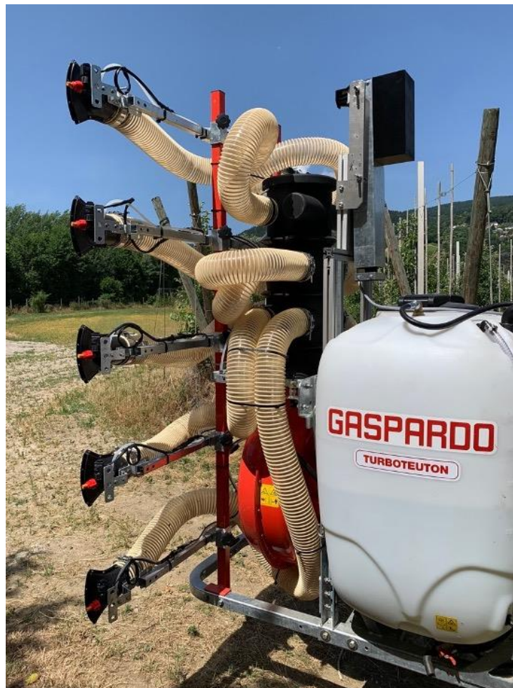
Figure 2: LiDAR-supported triggering system mounted on a state-of-the-art mist blower.
