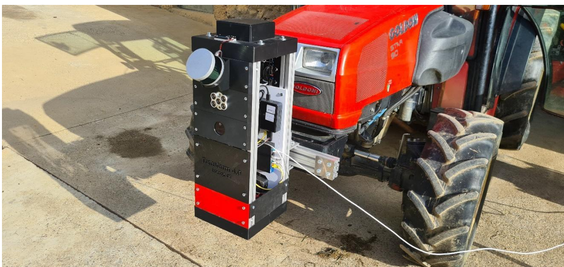
Figure 8 sensoric system mounted on the tractor
