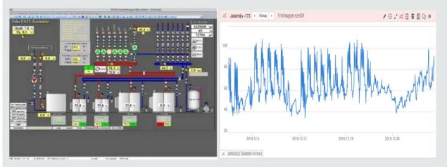
Dashboards are located in each measured buildings, usually at the entrance in order to reach the maximum possible number of persons in the building. The dashboards show the current consumption measured by the meters of the buildings (It differs from building to building: electricity is measured in all buildings, but at some buildings gas or heat consumption is also measured.). Curves of different time periods can be also visualized. The dashboards are not interactive.
