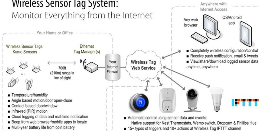
Picture 3: The topology of the system for indoor comfort measurement
