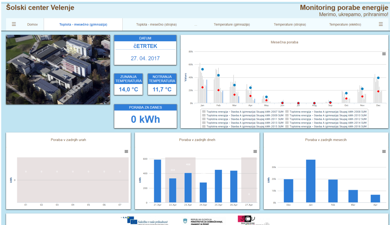
Figure 11: an example of DMS user interface which presents information data, data on monthly, weekly, daily, hourly and instantly energy consumption 10
