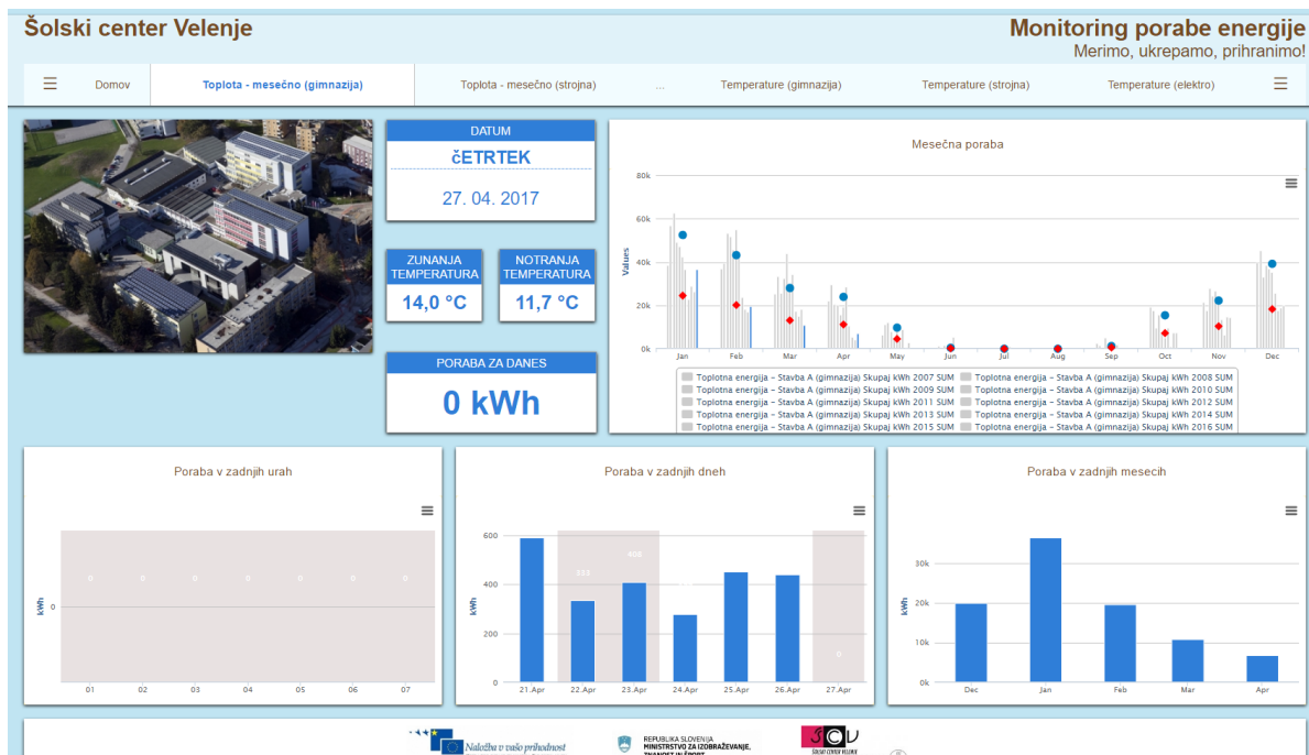
Figure 11: an example of DMS user interface which presents information data, data on monthly, weekly, daily, hourly and instantly energy consumption 11
