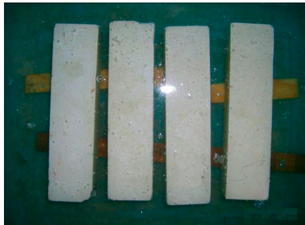
Photo 58. Investigation of water absorption of lime mortar at atmospheric. Soaking of samples.
