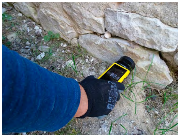
Photo 18. Moisture measurement by the microwave method
