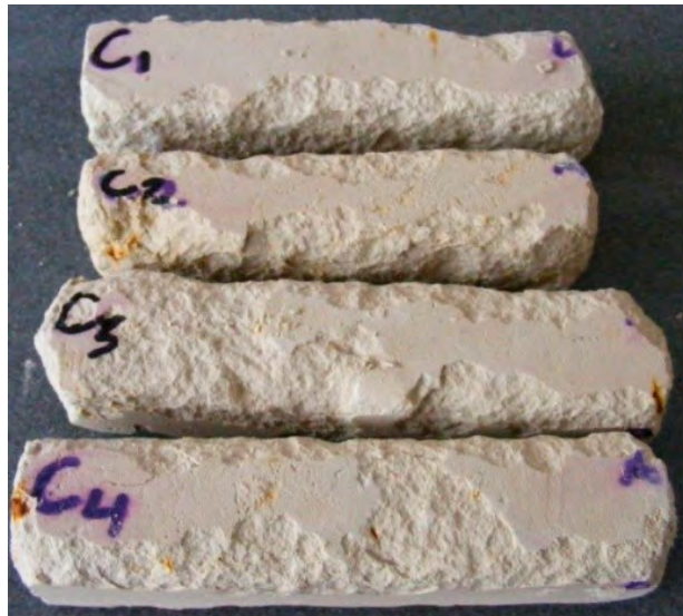
Photo 68. Frost resistance test. Samples from limestone rock after 56 freezing cycles.
