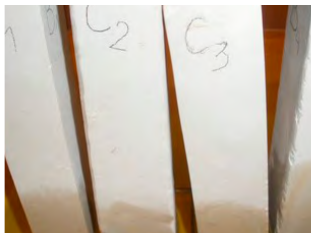
Photo 60. Determination of the capillary absorption coefficient for limestone rock. The end of the study.
