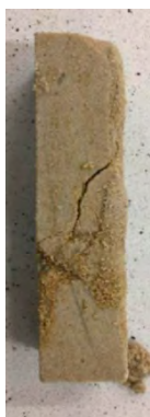
Photo 69. Frost resistance test. A sandstone sample after 30 freezing cycles. 4th degree damage
