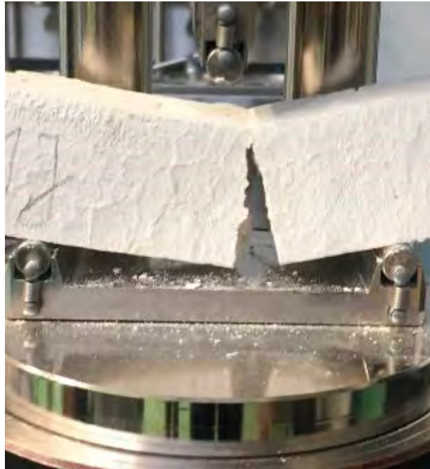
Photo 49. The process of testing a sample of conservation mortar in a strength testing machine.
