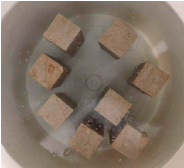
Photo 67. Frost resistance test. Soaking of sandstone samples.
