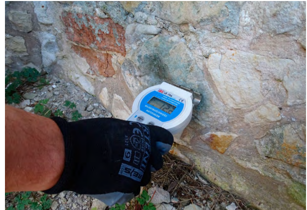
Photo 14. The LB-796 dielectric moisture meter.
