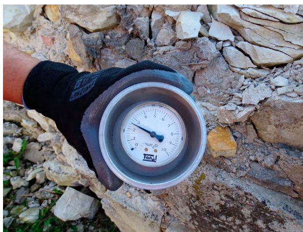
Photo 20. Investigation of moisture by the carbide method, reading of the acetylene pressure in the tank
