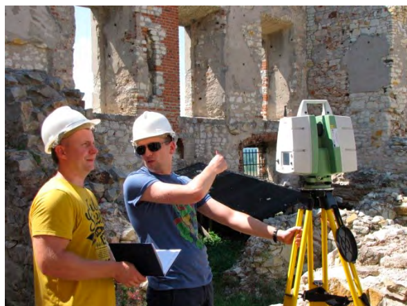
Photo 4. Leica ScanStation C10 while taking measurements
