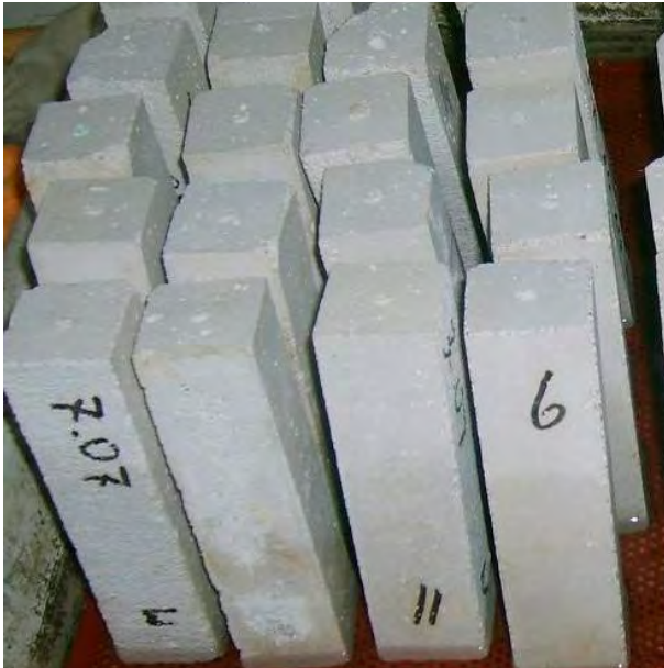
Photo 61. Determination of the capillary absorption coefficient for lime mortars. The beginning of the study.
