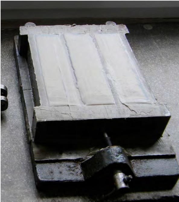
Photo 48. Mortar samples molding
