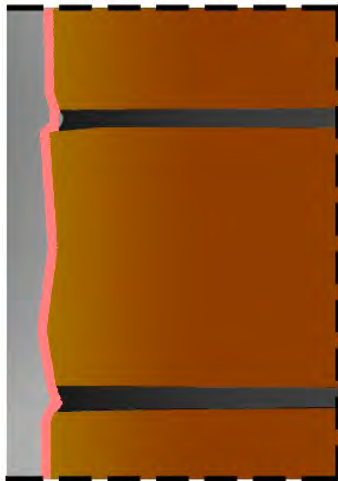
Figure 15. Salt corrosion at the interface between plaster and masonry
