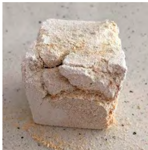
Photo 64. Resistance test for salt crystallization. Limestone rock samples after 10 cycles.
