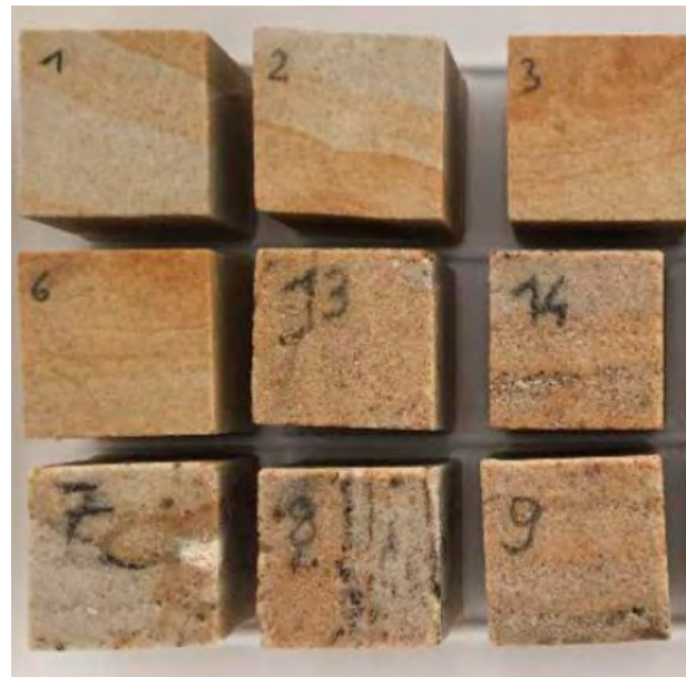
Photo 62. Determination of the capillary absorption coefficient for sandstone. The beginning of the study.
