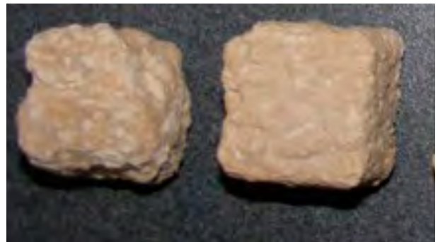
Photo 64. Resistance test for salt crystallization. Limestone rock samples after 10 cycles.
