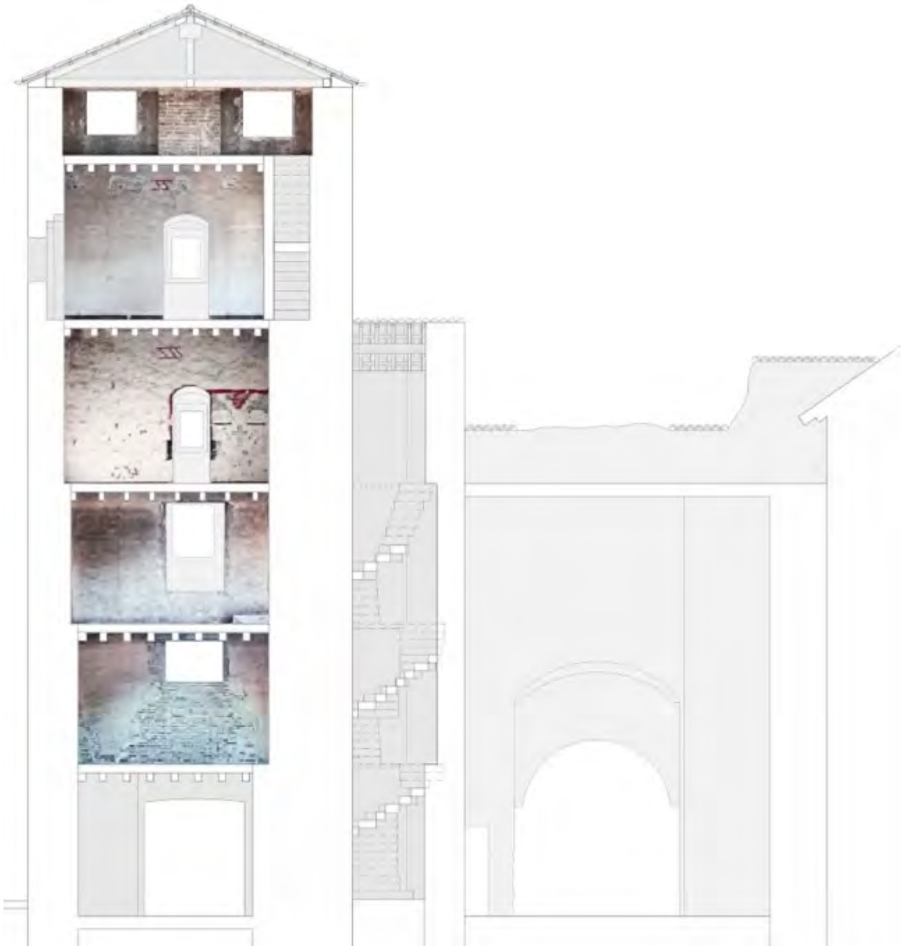
Image 3: Section with image showing straightening of internal walls
