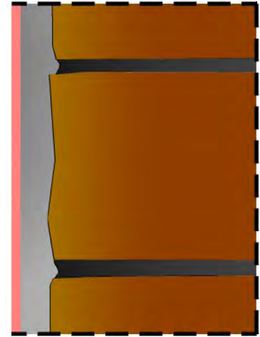
Figure 17. Salt corrosion on the surface of the plaster
