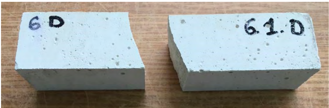
Photo 50. View of the sample after bending strength test.
