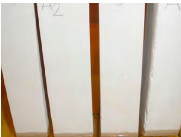
Photo 59. Determination of the capillary absorption coefficient for limestone rock. The beginning of the study.
