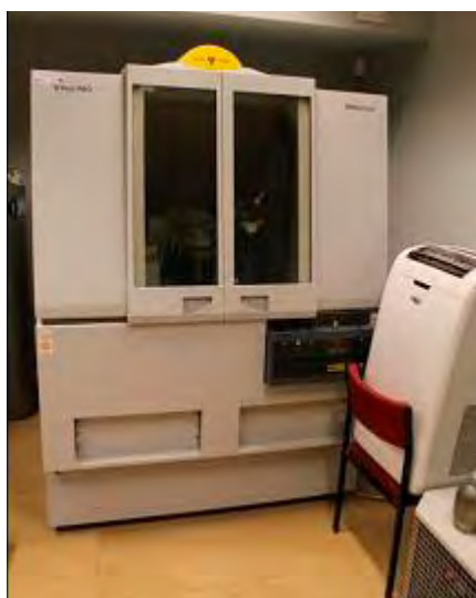
Photo 78. The X-ray diffractometer - X'pert PRO MPD by Panalytical. WBiA laboratory of Lublin University of Technology The XRD measurements of historical materials are made on powdered samples, the mass of sam-
