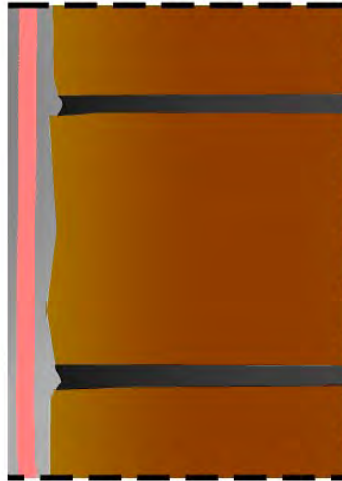
Figure 16. Salt corrosion inside the plaster layer
