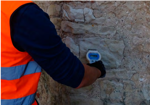
Photo 13. The LB-796 dielectric moisture meter.
