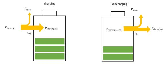
Figure 1: Visualization of a charging and discharging cycle of the storage
