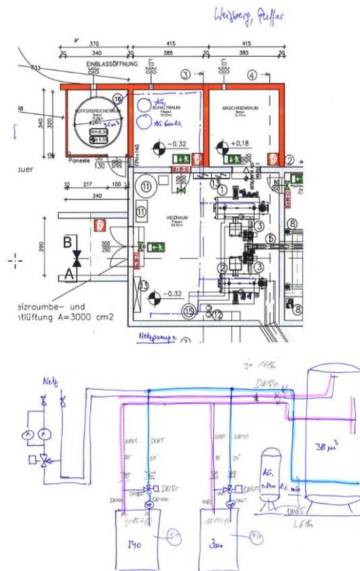
Figure 2: Scheme of the district heating station
