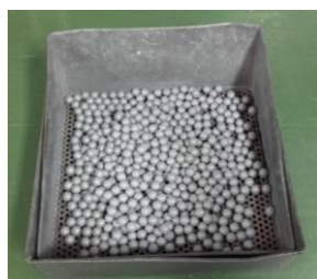
Figure 4 Three different charge made of balls of diameter 24, 15 and 10 mm
