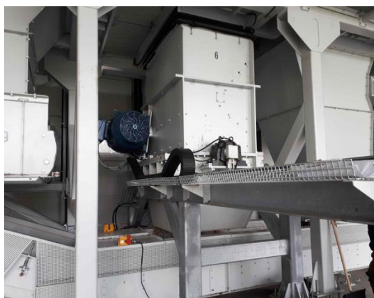
Figure 7. New hammer mill as pre-shredder
