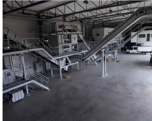
Figure 5. The drum sieve (back) and the KLME separator (front)
