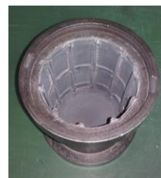
Figure 3 Ribbed inside surface of the mill
