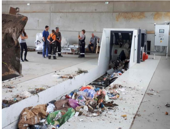
Figure 4. The moving floor conveyor and the bag opener
