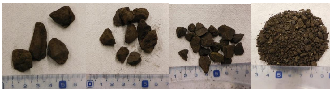
Figures 3., 4., 5. and 6. (from left to right) Bakonyoszlop slack coal (12.5–20 mm) sample, Bakonyoszlop slack coal (4–12.5 mm) sample, Bakonyoszlop coal dust (8–12.5 mm) sample, Bakonyoszlop coal dust (<8 mm) sample
