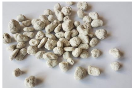
Figure 4 Aggregates produced from sewage sludge and glass waste (an own source)
