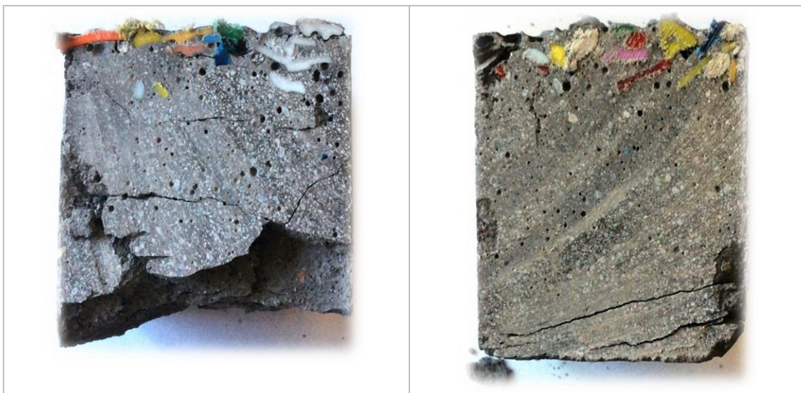
Figure 1 The irregular distribution of plastic particle in the geopolymer matrix, crosssection trough the samples after compressive strength test
