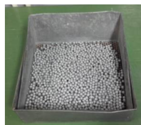
Figure 4 Three different charge made of balls of diameter 24, 15 and 10 mm
