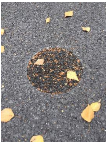
Figure 1: detector Installed at the spot with asphalt surface
