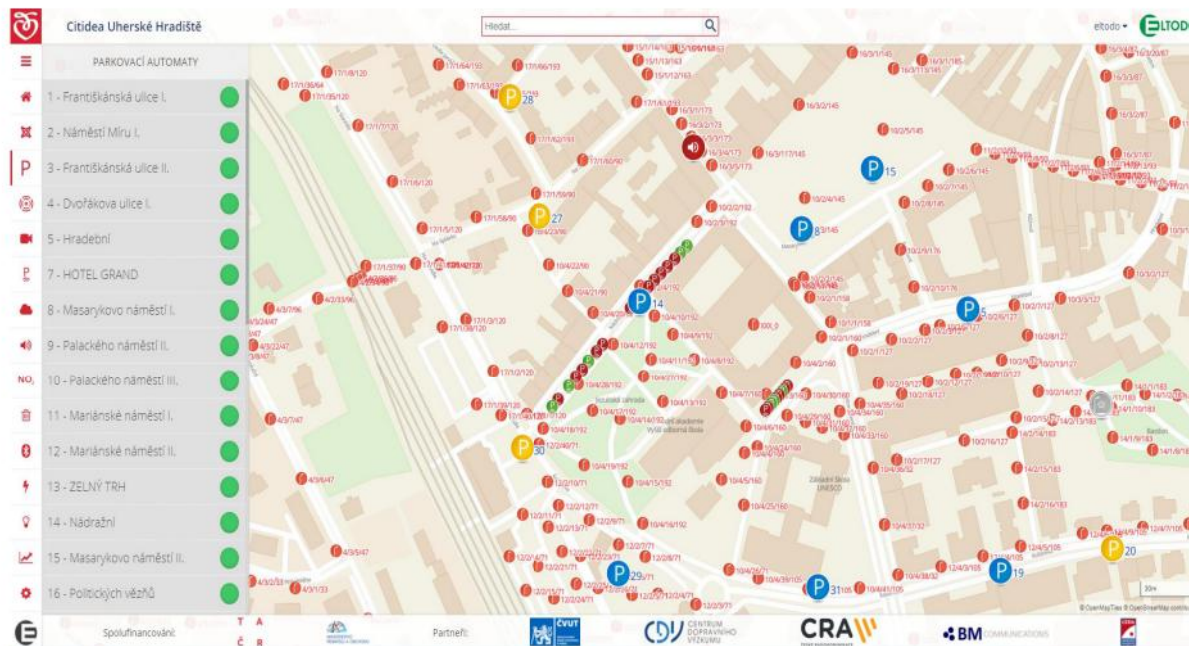
Figure 15: Integration platform of Smart Parking system including connected data from other sources (This is a SW result of the Czech R&D project Smartnet). SW provides visualization of parking data from various sources, i.e. sensors networks, payment terminals and shows the actual status of all the connected devices)
