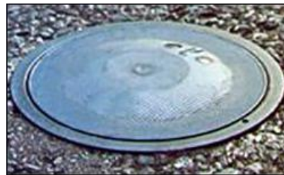
Figure 13: Infrared parking detector with integrated RFID (Westminster case)
