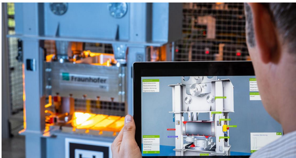
Figure 4 AR application visualizing current state of a Forming 4.0 presses
