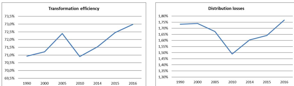
Fig. 27 Transformation efficiency (left) and distribution losses (right) in Germany in the time frame 1990-2016
