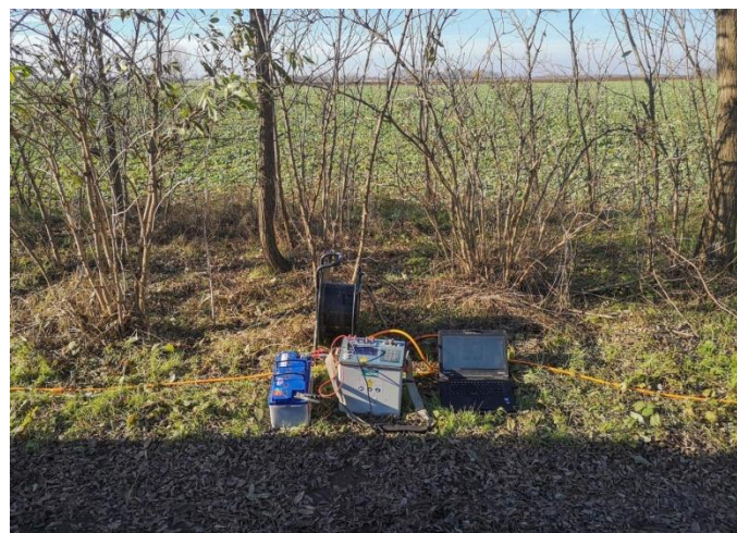
Geophysical geoelectric (ERT) measurements.
