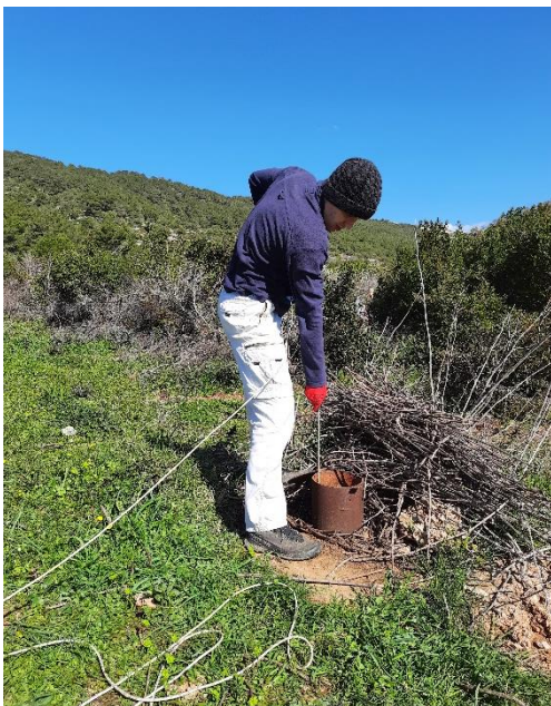
Groundwater level measurement.
