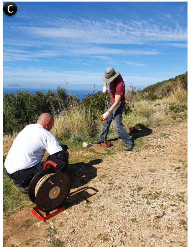
Fig.14. Field work in Croatia: A - water chemistry B - electrical resistivity testing C. groundwater table measurement
