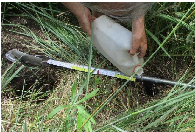
Fig. 19. Measurement of saturated hydraulic conductivity of soil by auger hole method (D.Vrablíková).
