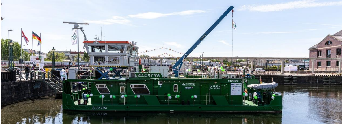
ELEKTRA-The first hydrogen driven pushboat. © BEHALA
