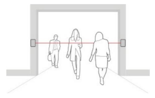
Fig. 26 - Horizontal infrared beam across an entrance, which counts persons passing through<sup>68</sup>.
