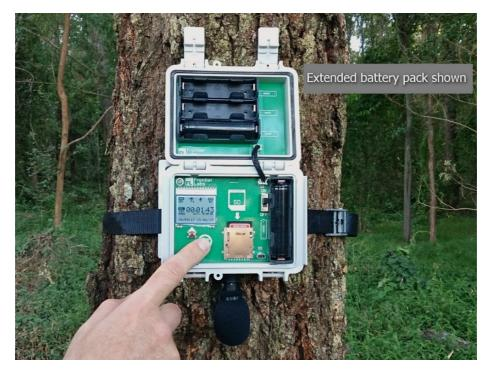
Fig. 44 - Example of installation of bioacoustics recording equipment 90.
