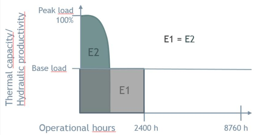
**Figure 58: Relation between energy content (E) and thermal capacity/hydraulic productivity shows that both parameters are necessary for a successful design of an open loop system.**
