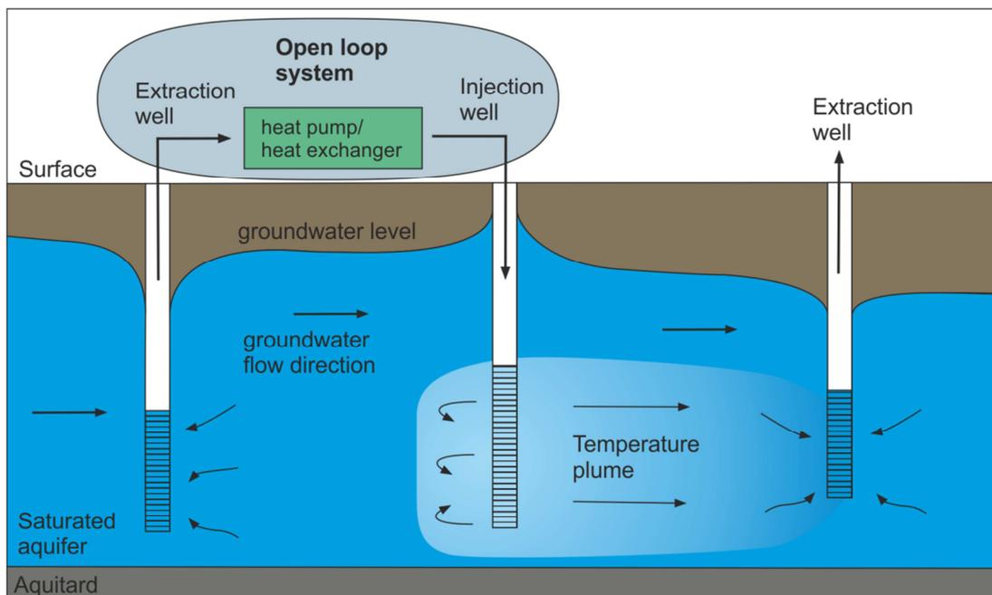
**Figure 56: Impact of open loop systems on extraction wells located downstream.**
