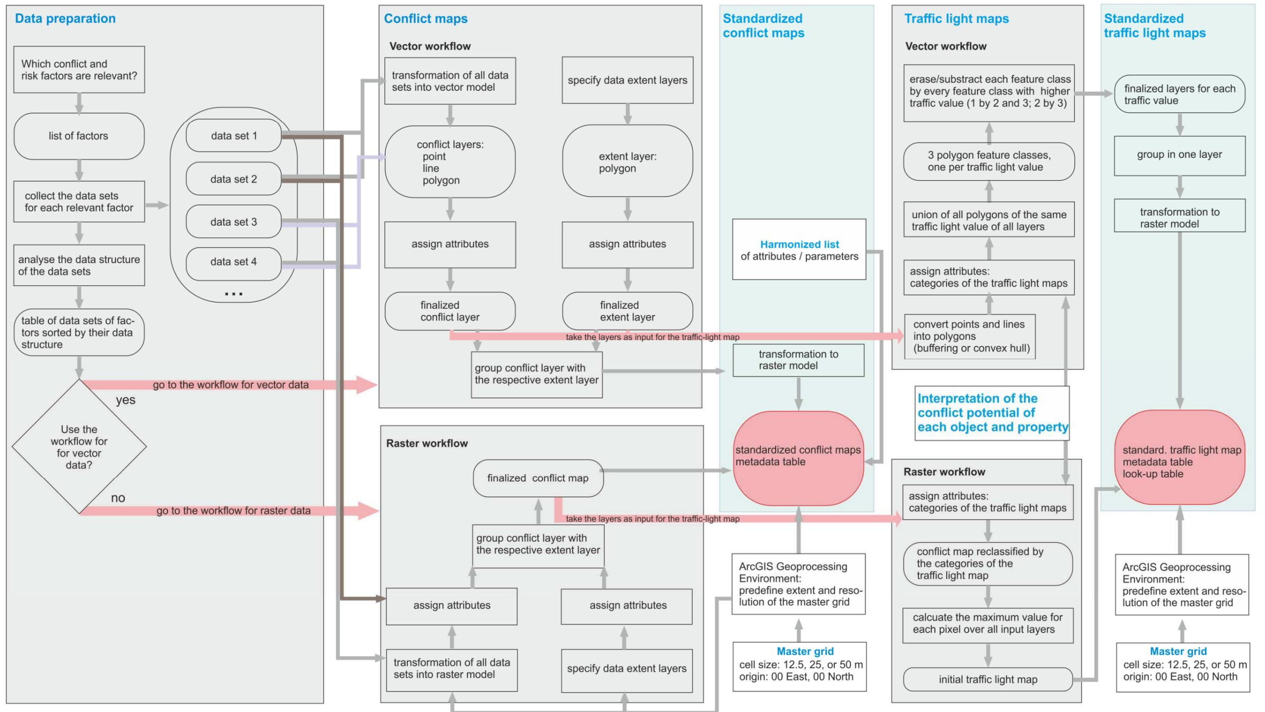
Figure 22: GeoPLASMA-CE workflow for mapping conflicts with shallow geothermal use and generating traffic light maps for the suitability of open or closed loop systems.
