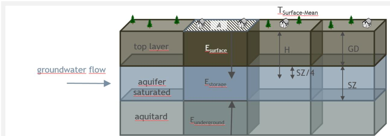
**Figure 57: Energy content for balanced use:  $E_{\text{storage}}$ . Energy content available for balanced use:  $E_{\text{surface}} + E_{\text{underground}} + E_{\text{storage}}$**
