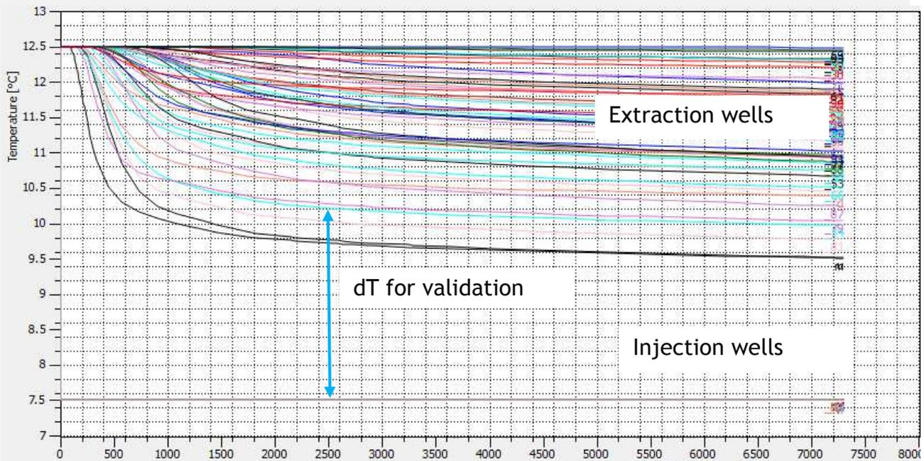
**Figure 59: Results of simulation. Temperature difference between extraction and injection well will be used to calculate the modelled energy content available. Temperature at injection wells remains constant**
