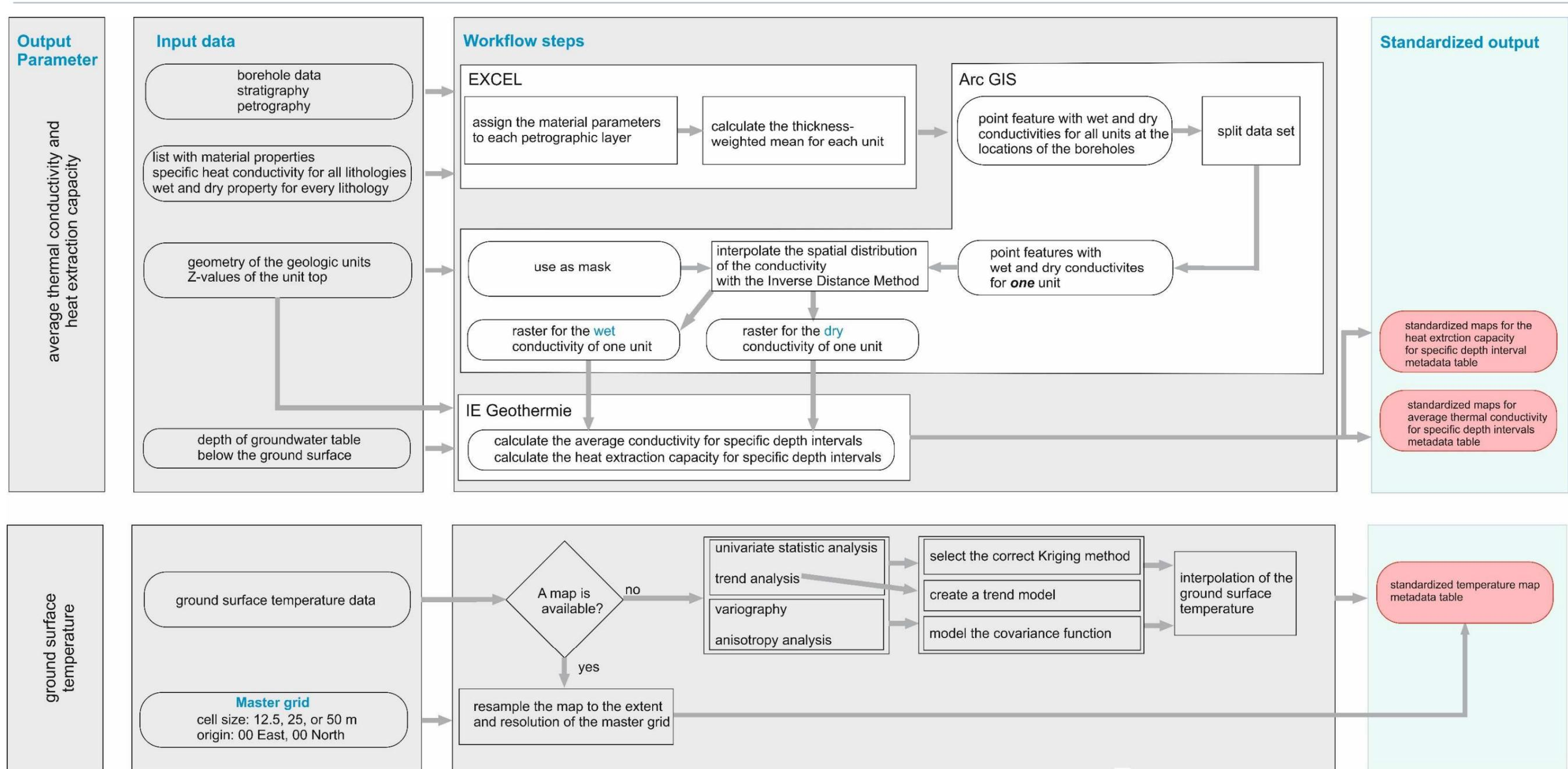
Figure 35: GeoPLASMA-CE workflow for mapping the geothermal potential for closed loop systems.
