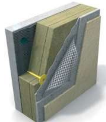
Figure 8: External thermal insulation composite systems
