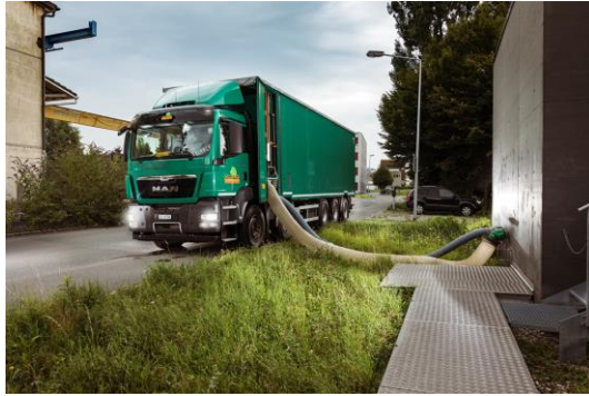
Figure 6.14 Pump container (source: Amstutz Holzenergie AG).
