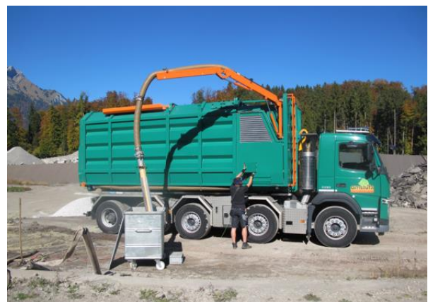
Figure 14.8 Transport vehicle with mounted ash extraction system (source: Holzenergie Schweiz).
