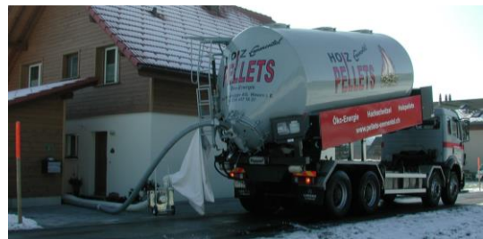
Figure 6.20 Pellets delivery with suction blower and dust bag (source: Holzenergie Schweiz)
