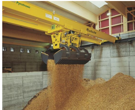
Figure 6.15 Fully automatic crane system with unloading trough and day silo (source: Schmid energy solutions).
