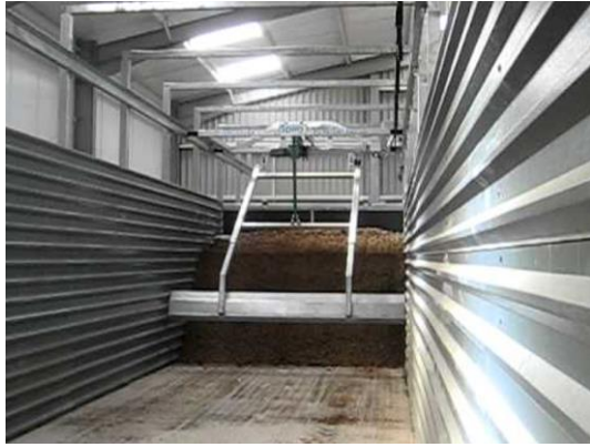
Figure 6.18 Top loader (source: Vecoplan AG).
