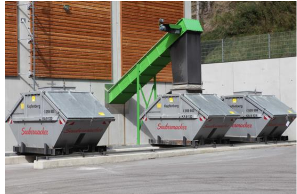
Figure 14.7 Ash trough changing device (source: AEE INTEC).
