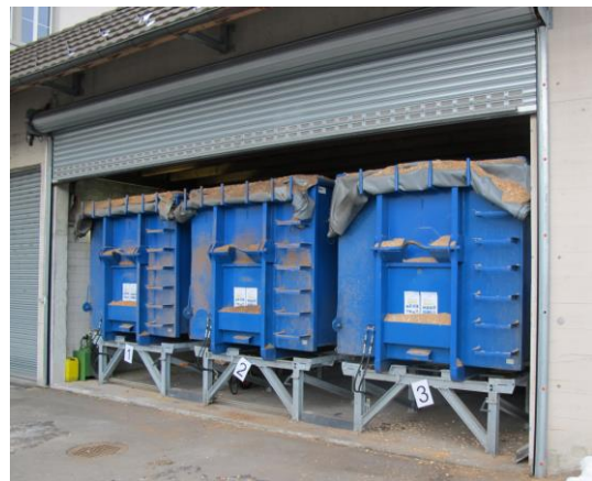
Figure 6.2 Mobile wood chips containers with discharge as a substitute for silos (source: Holzenergie Schweiz).
