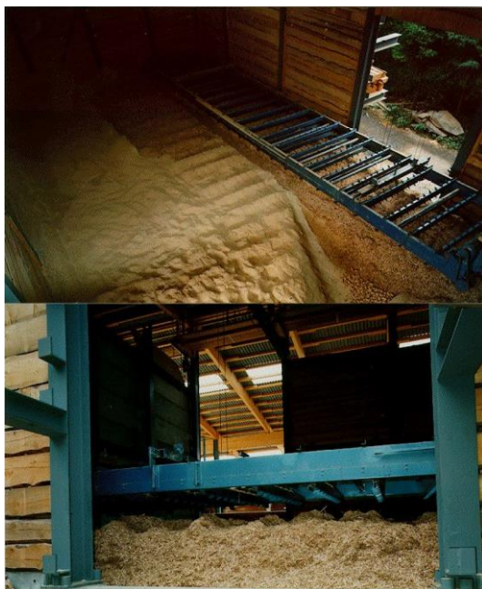
Figure 6.16 Loading and unloading system with horizontally and vertically movable scraper chain conveyor [68].
