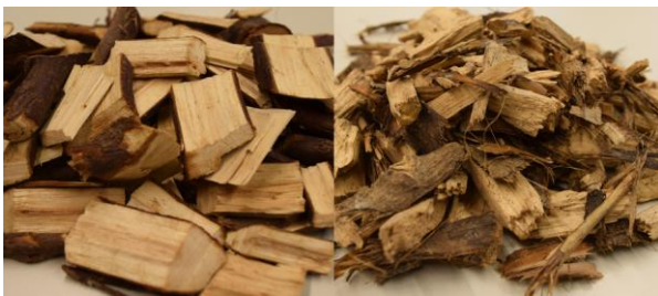
Figure 4.4 Differentiation between wood chips (cut with sharp tools, left) and shredded wood (chopped with blunt tools, right).
