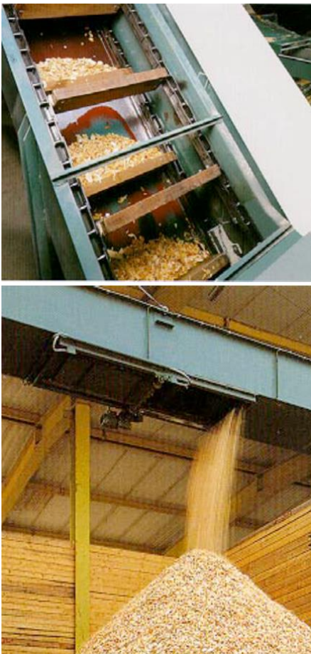
Figure 6.33 Scraper chain conveyor [69].
