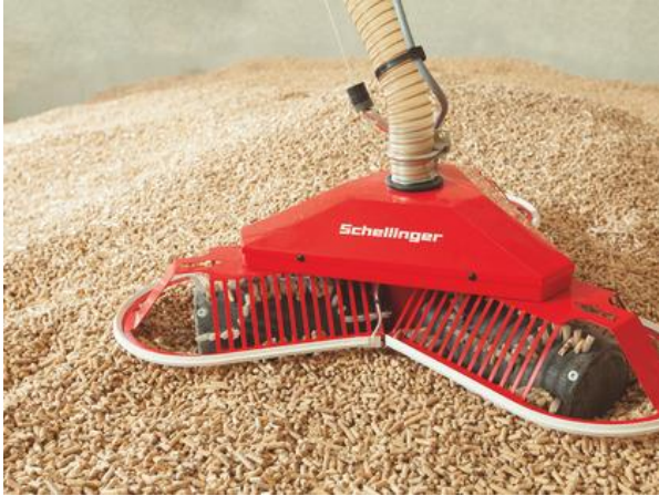
Figure 6.30 Pellet mole (source: Schellinger KG).
