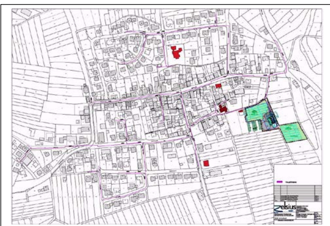
Network plan with heating plant
