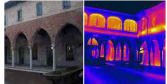
Thermographic mapping of an historic building's facade
