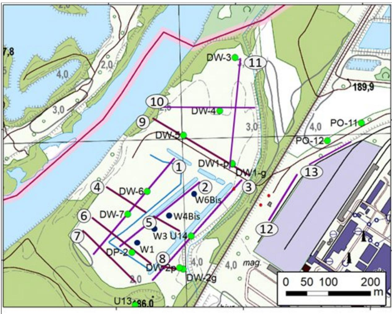
**Fig. 4. 14.** Location of 13 profiles obtained using electrical resistivity tomography (purple lines). Green dots represent location of the observation wells. Light purple area represent coal storage yard.
