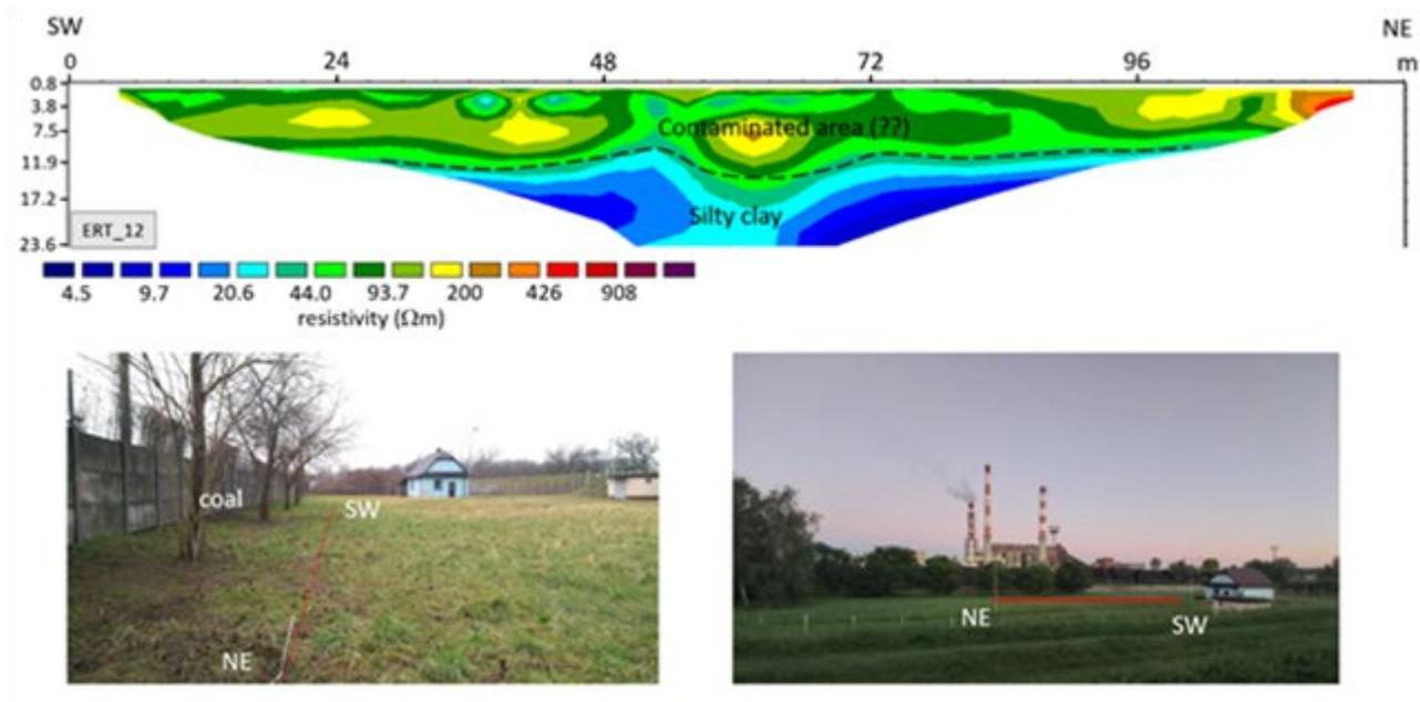
**Fig. 4. 17.** Inversion results of ERT<sub>12</sub> measurements conducted on the boundary with a coal storage yard of Grupa Azoty S.A.
