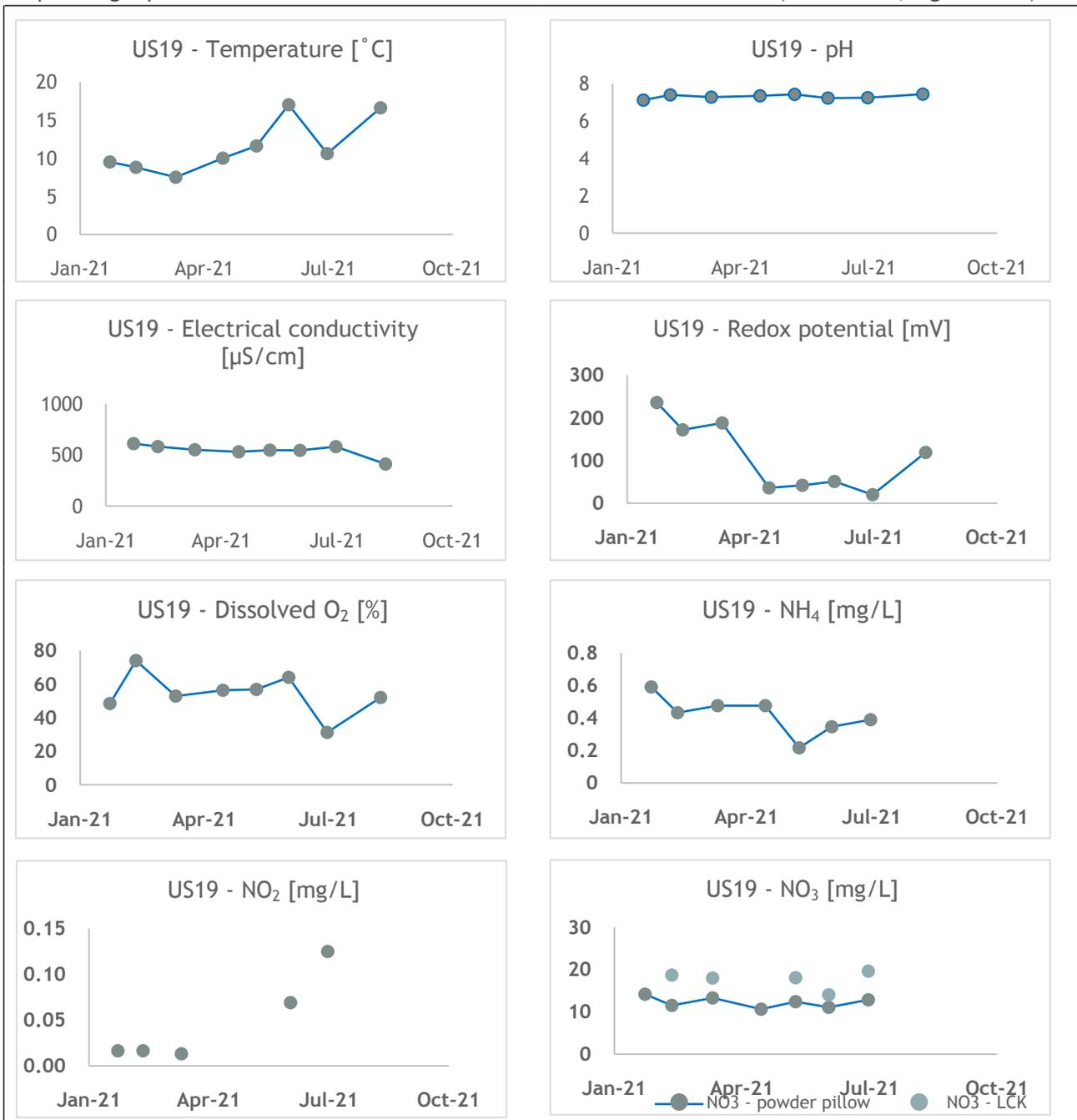
**Fig. 4. 27.** Time series of temperature, pH, EC, redox potential, dissolved O<sub>2</sub> and concentrations of NH<sub>4</sub>, NO<sub>2</sub> and NO<sub>3</sub> in the sampled groundwater from the abstraction well - US19.
