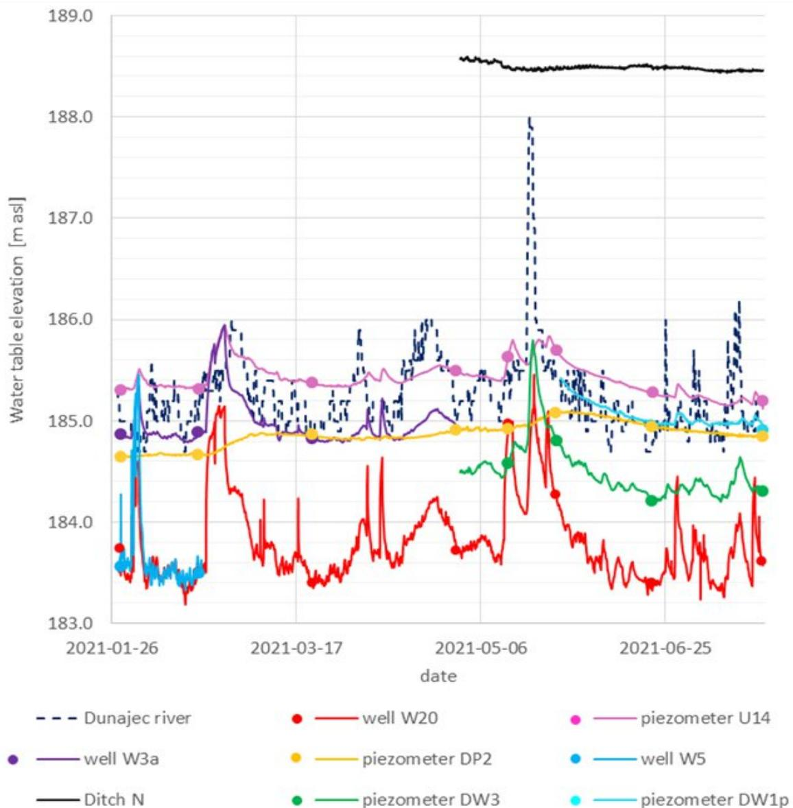
**Fig. 4. 23.** Water table elevation for selected observation points. Comparison of manual measurements (dots) with data from dataloggers (lines).
