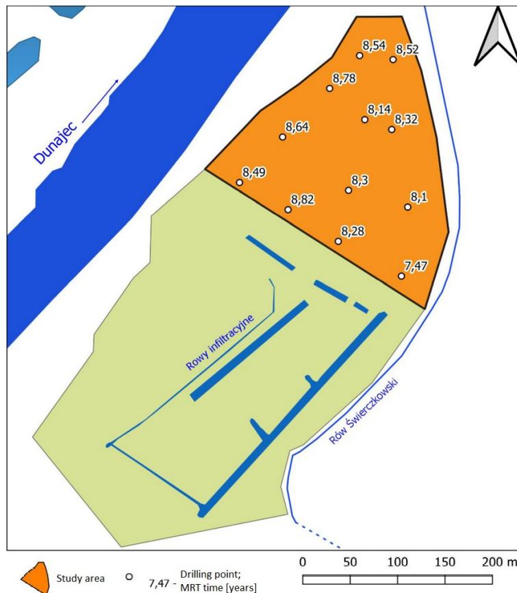
**Fig. 4. 18.** Calculated vertical seepage times (mean residence time of water MRT) through the unsaturated (vadose) zone in the northern part of the pilot site, as part of an engineering thesis (Bugla, 2021).
