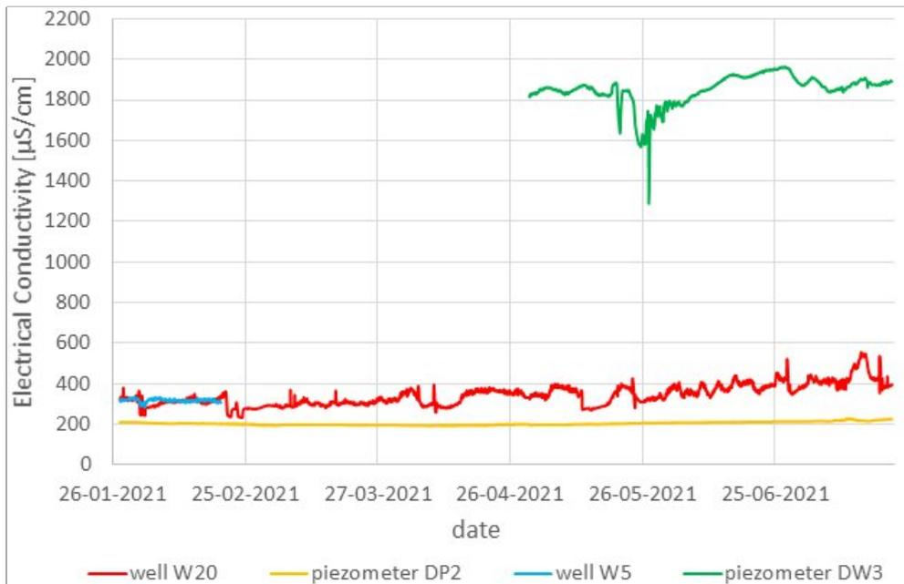
**Fig. 4. 26.** Electrical conductivity measurements at selected points at the pilot site.
