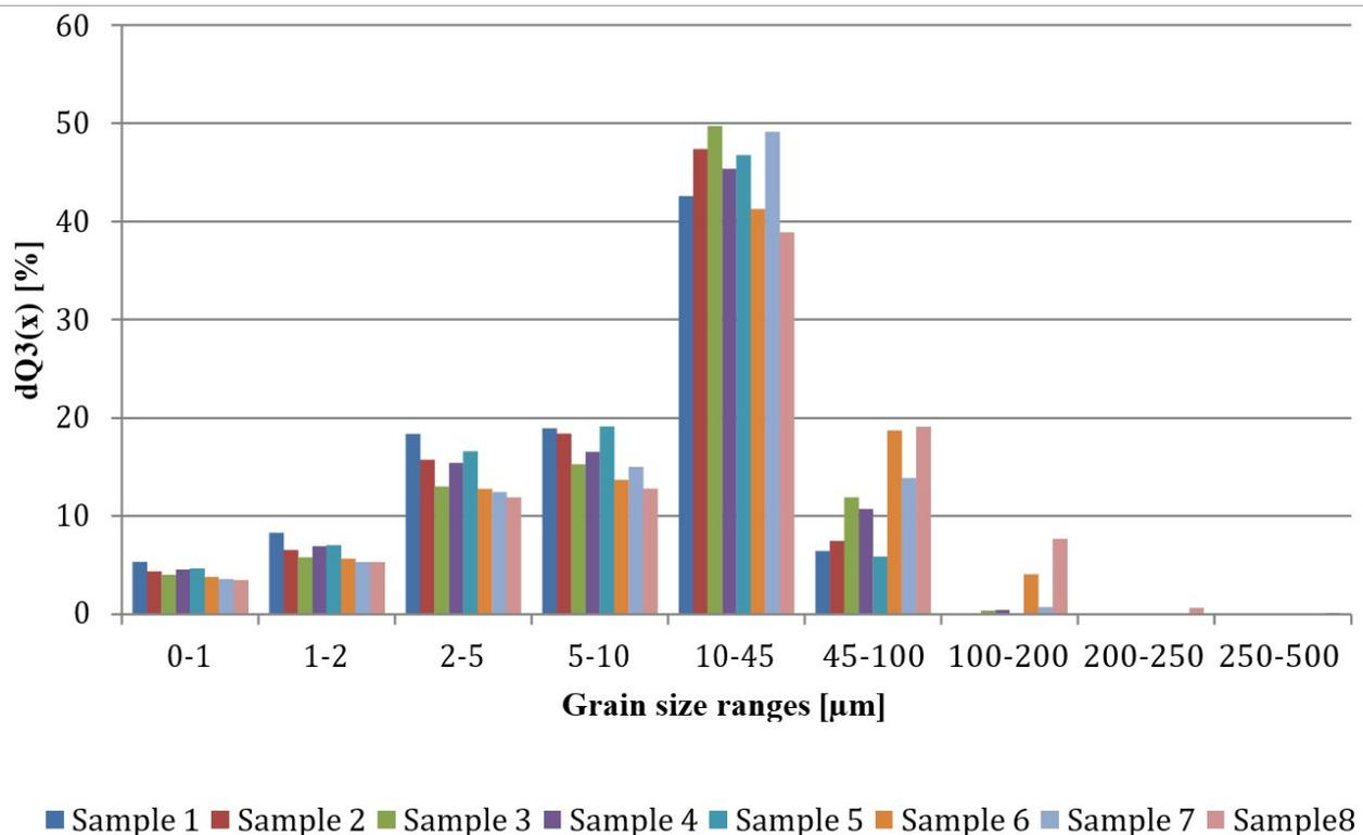
**Fig. 4. 19.** Percentage grain content of sediment samples from the bottom of infiltration ditches, determined with a laser particle analyser.
