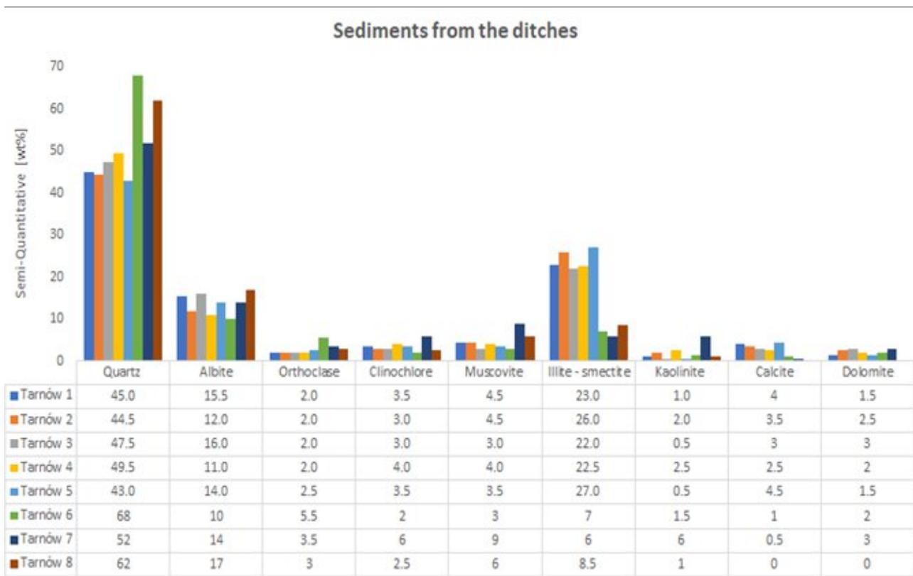
**Fig. 4. 20.** Results of XRD mineralogical analysis of 8 samples of bed sediments from the ditches.
