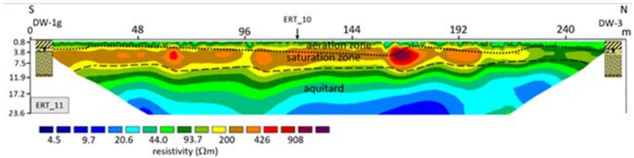
**Fig. 4. 16.** Inversion results of ERT<sub>11</sub> measurements and shallow boreholes conducted near ERT profiles at the potential MAR site. The hatched areas on the shallow boreholes from the top signify respectively for: DW-1g (soil, silt/sandy silt, loamy sand layered with pebbles, saturated gravel and pebbles with coarse sand, silty clay); DW-3 (soil, silt, loamy gravel with pebbles, saturated gravel with pebbles and coarse sand, clay).
