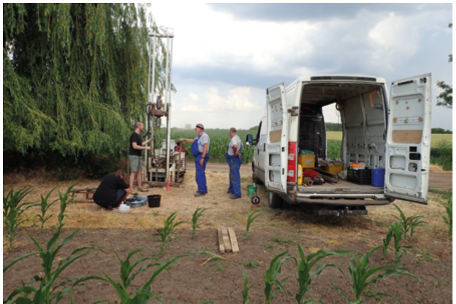
Geophysical Cone Penetration Test and groundwater sampling
