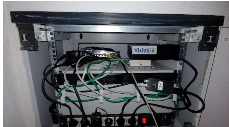
Fig. 11a,b - Three video-cameras system setting, placed on an existing pole (on the left), and the industrial PC embedding the software for images acquisition and processing with Artificial Intelligence features (on the top right of the right photo).
