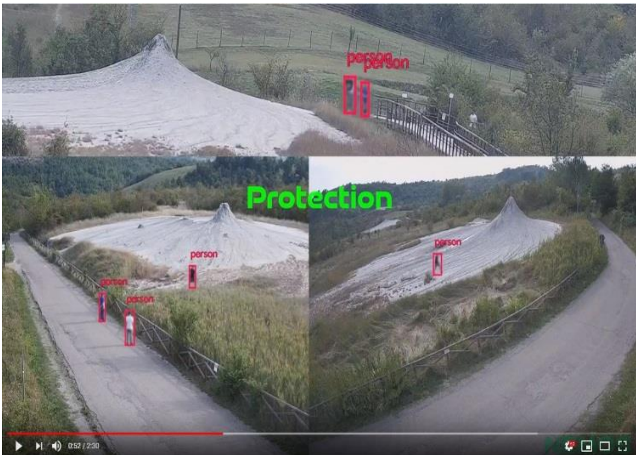
Fig. 14 - Testing phase of the system. Combination of the views of the three cameras, with the recognition of people walking on the street and invading the Zone A of the Natural Reserve, beyond the fences. From the entire explanation video: https://www.youtube.com/watch?v=6mbOOV_c0FI&feature=youtu.be .
