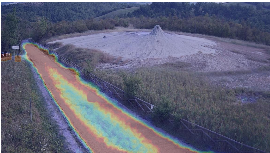
Fig. 28 - General HeatMap. As expected, the flow of vehicles and pedestrians, saturates the information along the municipal road. In any case it can be noted the splitting in two main parts, related to the go/back flows.
