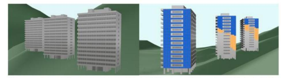
βD representation of the three high rise buildings; (right) representation of the BIPV plant with two optimal NPV solutions: if the cost of storage is 1000 €/kWh no battery is <u>installed</u> and the plant is limited at the blue area. If the cost of storage is 250 €/kWh, 87 kWh of batteries are installed allowing a larger BIPV plant (orange area).
