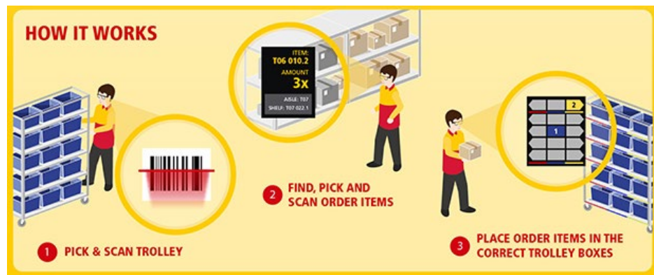
Figure 1 - Augmented reality supported picking in DHL warehouse [3]
