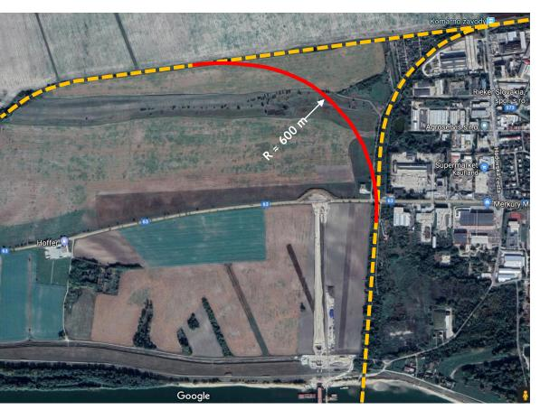
Triangle track could be built west of Komárno station over open field
