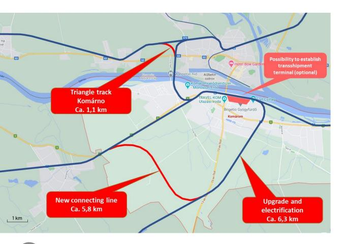
Triangle track Komárno in combination with connecting line south of Komárom would avoid changes of travelling direction in all traffic relations!
