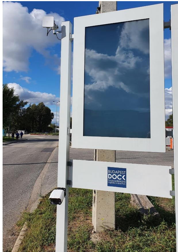
2. Figure: Tailor-made screen of the smart system equipped with license plate recognizing camera and Wi-Fi antenna
