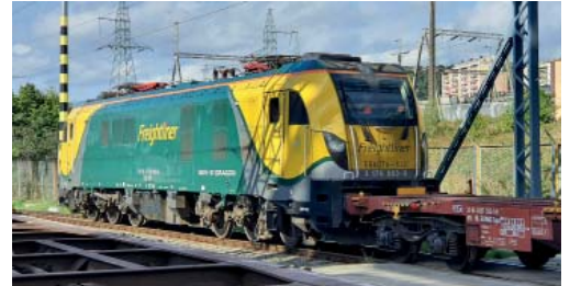
■ Freightliner PL's Dragon locomotive with its flexible diesel electric design and onboard I.T./GPS also represents a step forward for intermodal rail – seen here at BCT in October
