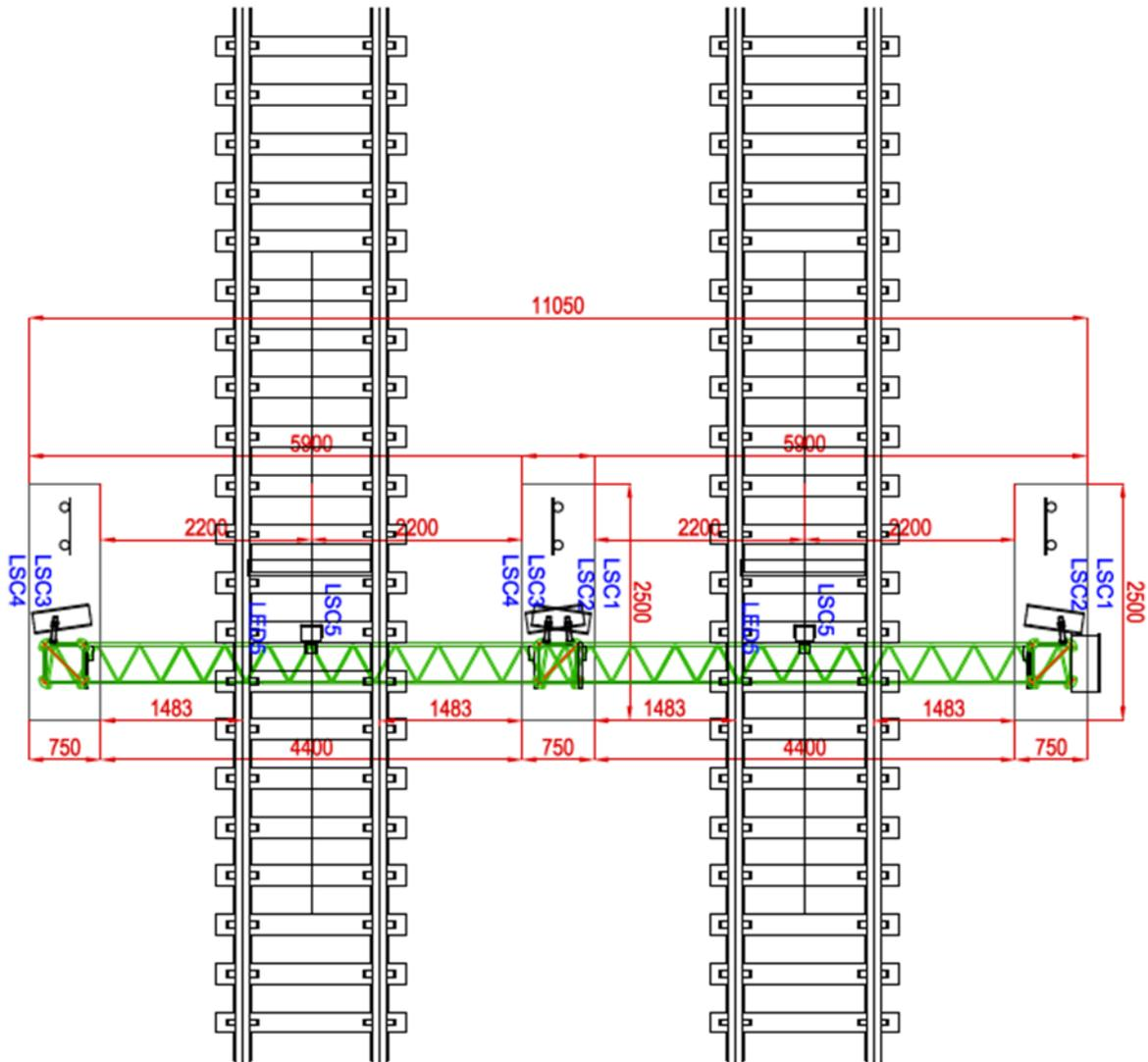
Figure 2: design of the OCR system in the port of Koper (Source: Luka Koper's archive)
