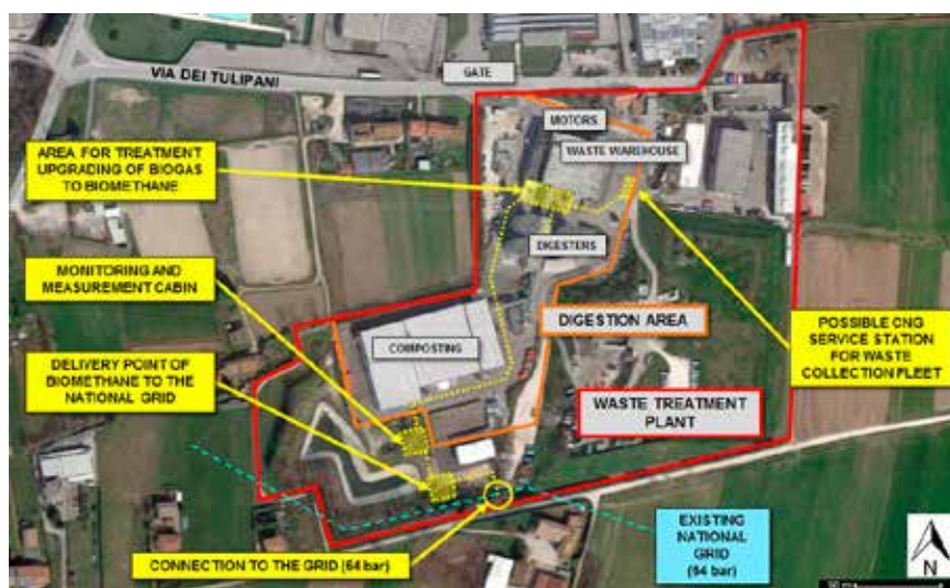
Figures 3.4: ETRA's plant in Bassano del Grappa (right) and biomethane production (left)
