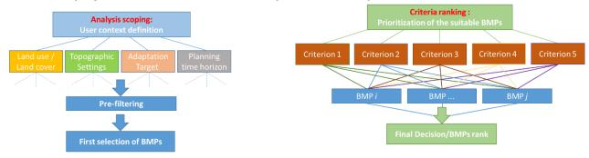
**Figure 1:** Schematic representation of the GOWARE structure. The pre-selection of BMPs is shown on the left side while the BMPs prioritization is shown on the right side.
