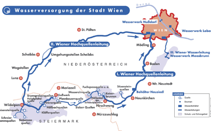
Figure 31: Water supply of Vienna with the two main transport pipelines (I. and II. Wiener Hochquellenleitung) from the Pilot areas.
